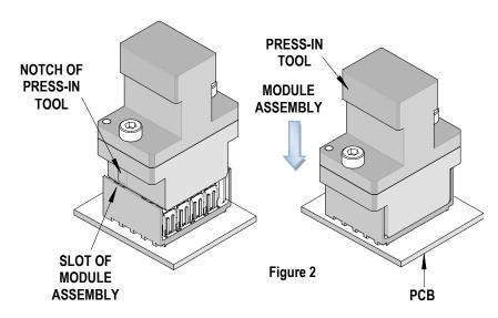
appropriate press, seat the header assembly until there is less than 0.10mm (.004 in) clearance between the bottom of the plastic housing and the surface of the PCB. See Figure 3.
