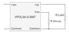
Figure 12. Trim-up Voltage Setup
