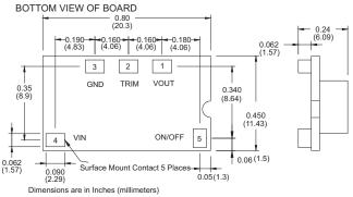
Dimensions are in inches (millimeters) Tolerances :x.xx  $\pm$  0.02in.( x.x  $\pm$  0.5mm) , unless otherwise noted x.xxx  $\pm$  0.010in. ( x.xx  $\pm$  0.25mm)
