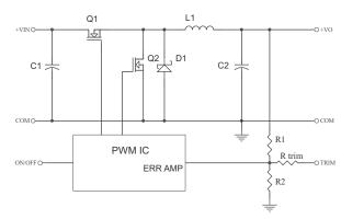
Figure 1. Electrical Block Diagram
