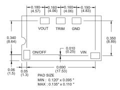
Figure 5. Recommended SMT Footprint (Top View)
