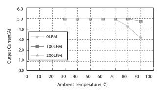
Figure 3. Typical Power De-rating for 5V IN 3.3Vout
