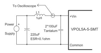
Figure 10. Input Reflected-Ripple Test Setup
