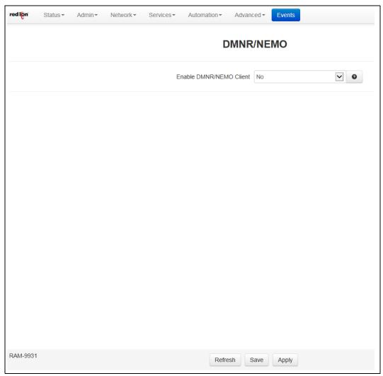
**Enable DMNR/NEMO Client:** Yes/No options to enable a DMNR/NEMO client (Dynamic Mobile Network Routing / Network Mobility).
