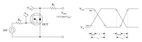
Fig 14. Unclamped Inductive Switching Test Circuit & Waveforms
