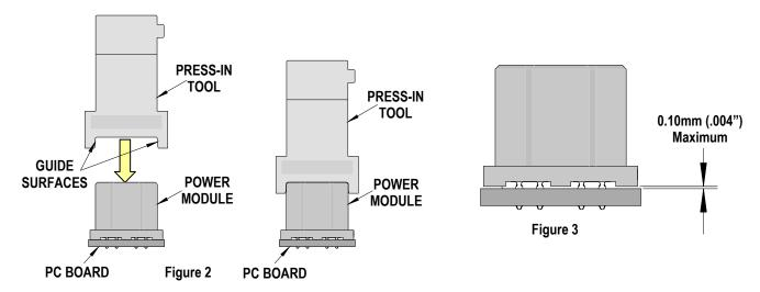
3. Using the application tool and an appropriate press, seat the vertical power module until there is less than 0.10mm (.004 in) clearance between the bottom of the plastic housing and the surface of the PCB. See Figure 3.
