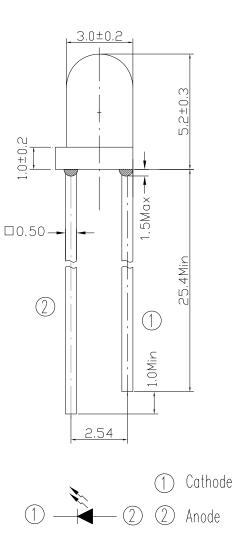
Note: Tolerances unless dimensions ±0.25mm
