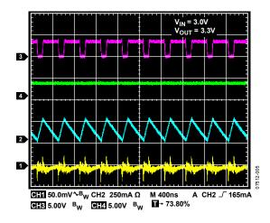
Figure 5. Boost Operation,  $V_{IN} = 3.0 V$ ,  $V_{OUT} = 3.3 V$ ,  $I_{LOAD} = 500 mA$ , PWM
