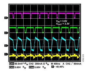
Figure 6. Buck Operation,  $V_{IN}$  = 4.0 V,  $V_{OUT}$  = 3.3 V,  $I_{LOAD}$  = 500 mA, PWM
