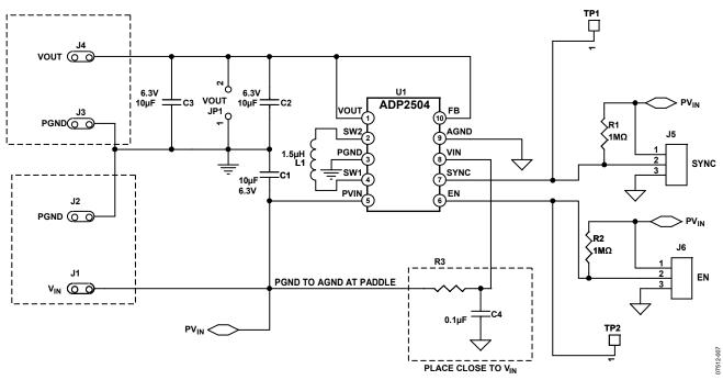
Figure 8. ADP2504 Evaluation Board Schematic
