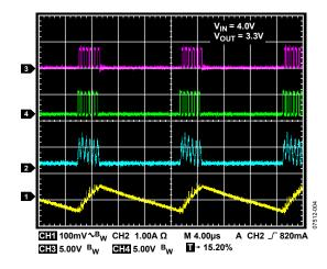
Figure 4. Buck Boost,  $V_{IN} = 4.0 V$ ,  $V_{OUT} = 3.3 V$ ,  $I_{LOAD} = 50 mA$ , PSM
