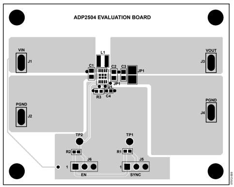
Figure 9. Top Layer, Recommended Layout
