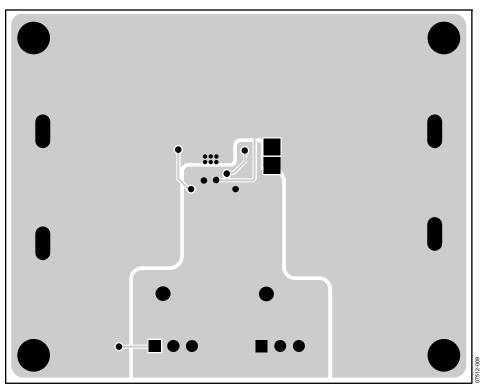
Figure 10. Bottom Layer, Recommended Layout
