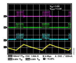
Figure 3. Buck Boost, V<sub>IN</sub> = 3.0 V, V<sub>OUT</sub> = 3.3 V, I<sub>LOAD</sub> = 50 mA, PSM
