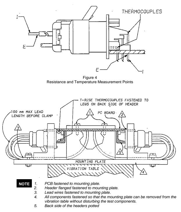
Figure 5 Vibration and Physical Shock
