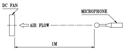
NOISE IS MEASURED AT RATED VOLTAGE IN FREE AIR IN ANECHOIC CHAMBER WITH B & K SOUND LEVEL METER WITH MICROPHONE AT A DISTANCE OF ONE METER FROM THE FAN INTAKE.
