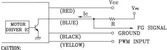
THE LEAD WIRE OF FG SIGNAL CAN NOT TOUCH THE LEAD WIRE OF POSITIVE OR NEGATIVE.
